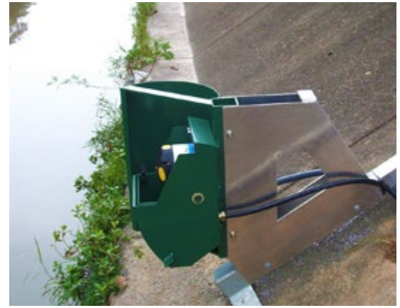
Innovative “Knights Head” stations use automatically retracting hoods to protect SonTek Argonaut current meters.
